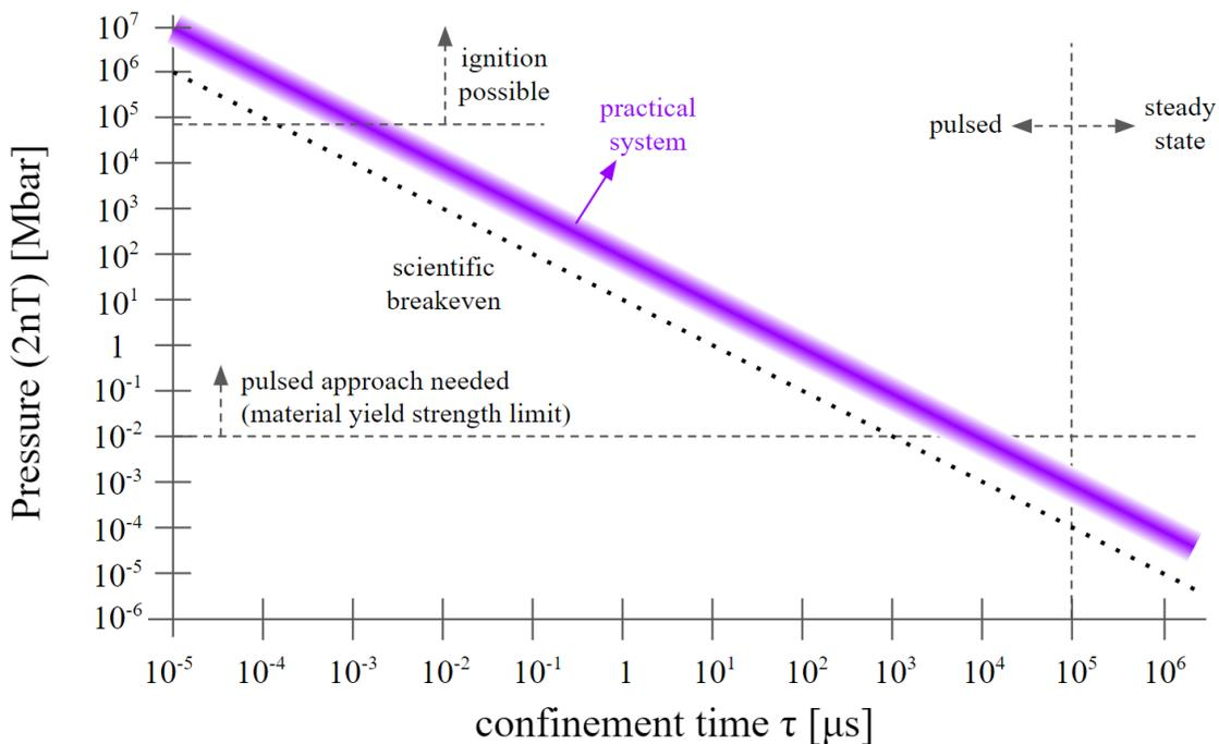
**Fig 3:** To achieve a good fusion burn and net-positive gain, a practical D-T fusion energy system must achieve a sufficiently high value of the Lawson product  $P\tau$  (at a temperature of at least  $\sim 10$  keV).  $P\tau$  thresholds for scientific breakeven ( $\sim 10$  bar-s) and practical systems (30-100 bar-s) are shown above.
