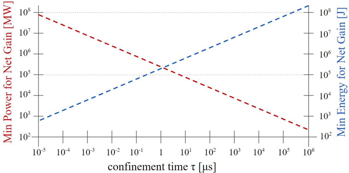
**Fig 4:** Estimated minimum energy and minimum power for fusion systems that can achieve net gain, scaling from a  $Q > 1$  tokamak (200 MJ plasma energy, 200 MW heating power), a rough average of ITER and CFS designs. Real concepts will depart from this curve owing to different methods of heating/confinement, but this estimate is a reasonable proxy for magnetic confinement which can be utilized (steady-state or pulsed) across the full timescale spectrum.
