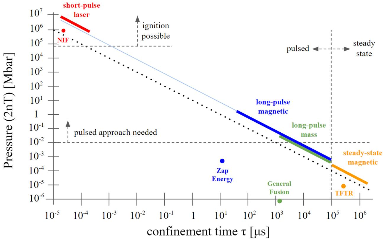
**Fig 7:** Estimated experimentally-demonstrated  $P\tau$  (solid dots) for various D-T approaches, relative to  $P\tau$  needed for practical systems (solid colored lines) and for  $Q > 1$  (dotted line). The TFTR tokamak achieved [P \$\tau\$  ~ 2.5 bar-s](#).
