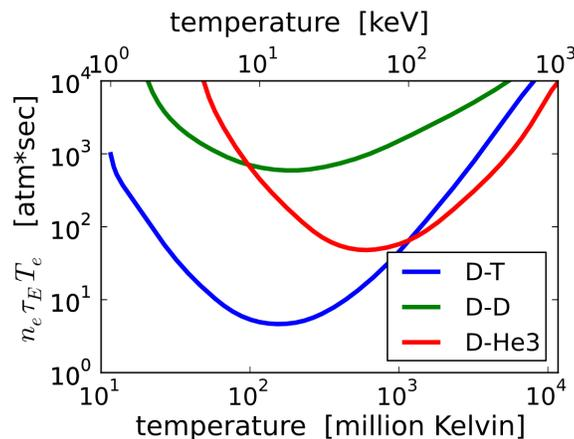
**Fig 2:** For a given fuel, the Lawson criterion is derived by finding the threshold  $L = nT\tau$  at which the power released in charged byproducts exceeds the input power needed to sustain the plasma burn. For D-T, one must achieve  $P\tau \geq 10$  bar-second at  $T \sim 10^8$  Kelvin. (Plot is from [Wikipedia:Lawson Criterion](#).)
