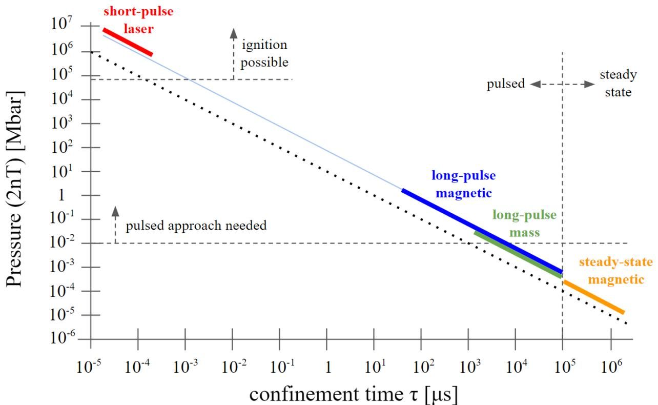
**Fig 6:** Practical  $P\tau$  needed to achieve system-relevant gain ( $Q_{\text{facility}} > 1$ ) for four types of D-T systems (solid colored lines), relative to  $P\tau$  for scientific breakeven ( $Q > 1$ , dotted line).
