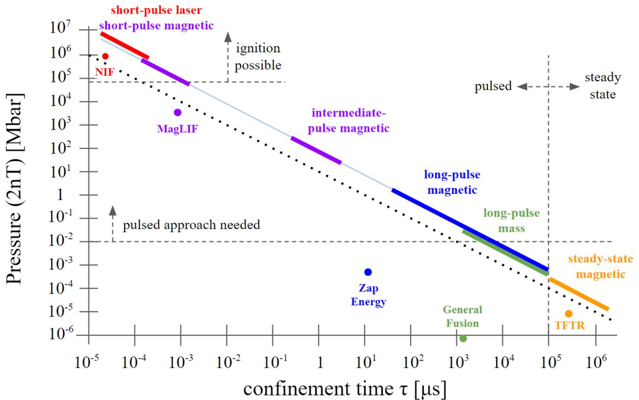
**Fig 8:** This Figure adds the short-pulse magnetic (Magnetic Igniter) and intermediate-pulse magnetic (Sweet-Spot Burner) regimes to Figure 7, and includes recent MagLIF performance, as discussed below.
