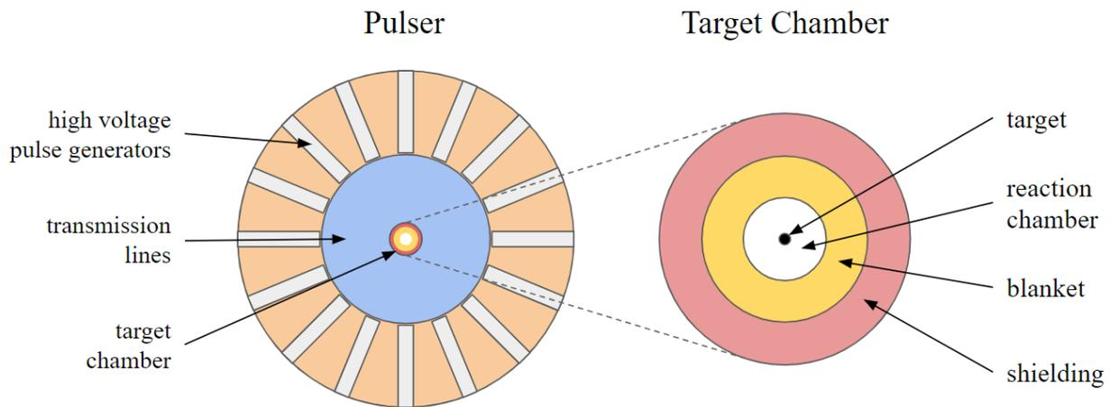
**Fig 9:** This top-down sketch shows elements (not to scale) of a pulsed magnetic fusion system: (1) a pulser made of high voltage pulse generators that drive energy pulses down transmission lines to the target, and (2) a target chamber with a target inside a reaction chamber, surrounded by a blanket and shielding. In a commercial system, the blanket would capture heat and transfer it to an energy conversion system to utilize the energy released.
